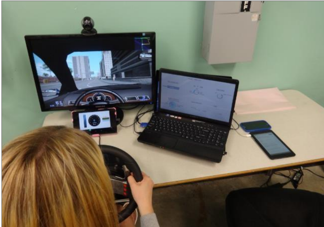
Figure 18 The setup; Driving simulator window, standard display in front of steering wheel, secondary displays, tablet for entering probe answers and scales, and a phone for stopwatch & timing.
