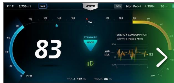
Figure 2 Digital speedometers like the one above from Mission Motorcycles are increasingly common. The curved orange bar on the right denotes battery output; when acceleration increases the wattage output increase is shown by the orange bar moving upward. When the driver decelerates the bar goes below 'zero' and represents regenerative energy.
