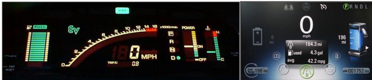
Figure 7 The appearance of digital displays, with differently style graphics, digital numeric, and 3d visualizations is quite the departure from previous instrument cluster design conventions. Source: Nissan Altra and Chevy Volt.
