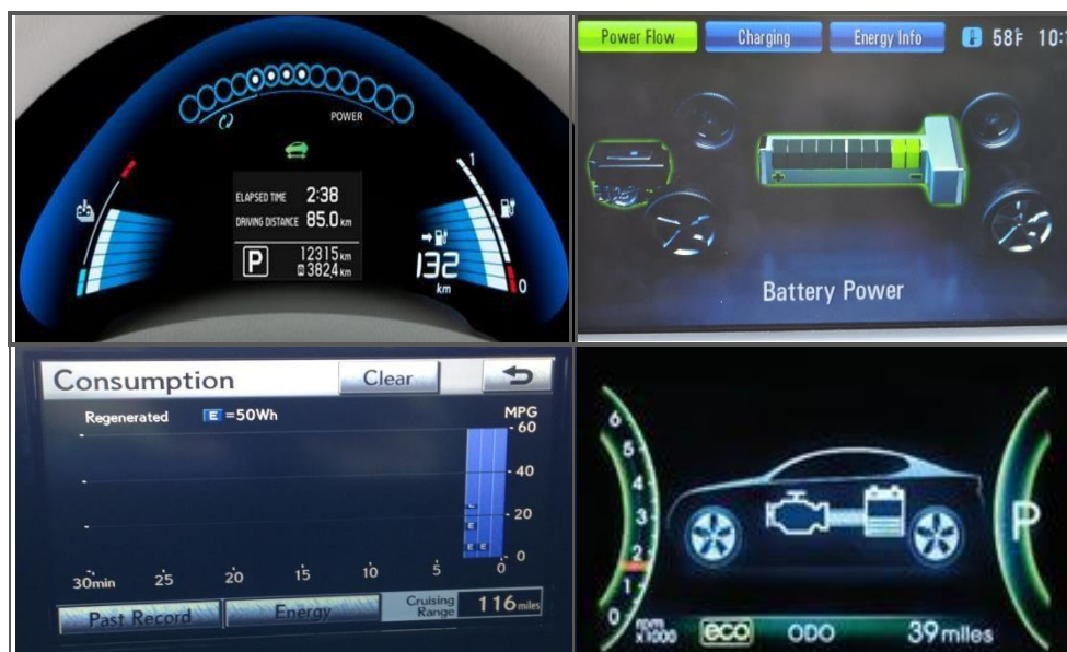
Figure 8, [From top left, clockwise] a) The Nissan Leaf employs a circular array that contains four filled dots that move right for output and left when regenerative braking is activated. b) The Chevy Volt 'power flow' screen, c) The Lexus CT consumption screen showing regenerated power, d) the Kia Hybrid active regenerative braking graphic.
